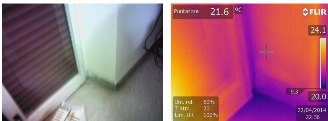
FIGURE 232 - THERMAL LOSSES IN THE WINDOWS AND WINDOW INVISIBLE TO THE NAKED EYE
