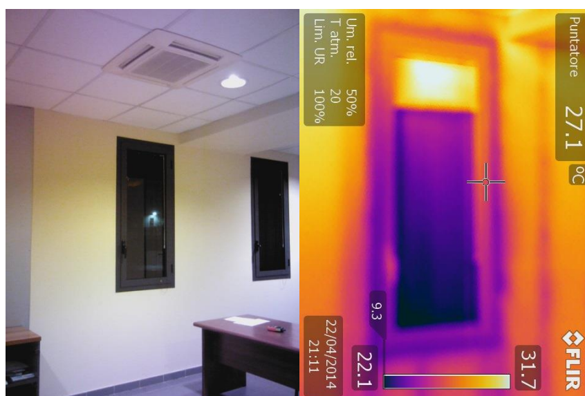
FIGURE 40 - THERMAL LOSSES IN THE WINDOWS AND WINDOW INVISIBLE TO THE NAKED EYE
