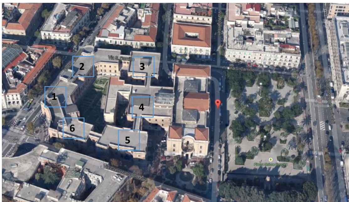
FIGURE 185 - SIX AREAS AVAILABLE FOR THE PV SYSTEM INSTALLATION
