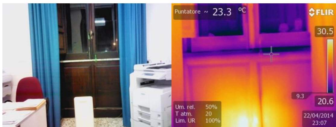
FIGURE 148 - THERMAL LOSSES IN THE WINDOWS AND WINDOW INVISIBLE TO THE NAKED EYE
